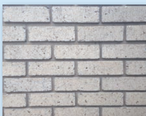
CEMENT STOCK BRICK
